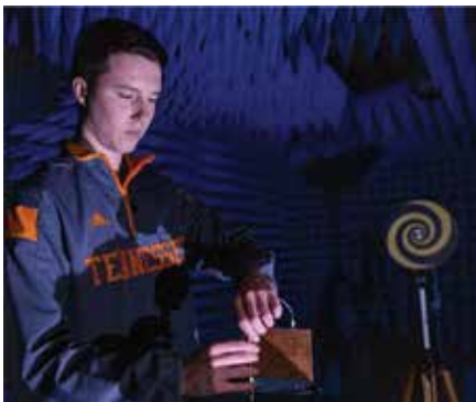
UT graduate student Chandler Bauder examining a wideband antenna for testing in an anechoic chamber that will be used extensively in the proposed 5G antennas evaluation.
